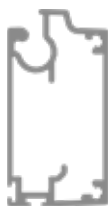
Heavy 28 x 54,9 mm Extra weight. Advised at widths and heights > 3 m. Extra stability to wide screens.
