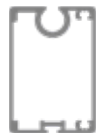
Heavy 28,6 x 41,9 mm Extra weight. Advised at widths and heights > 3 m. Extra stability to wide screens.
