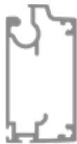
Heavy 28 x 54,9 mm Extra weight. Advised at widths and heights > 3 m. Extra stability to wide screens.
